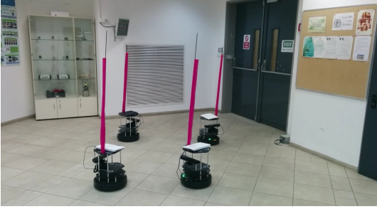
(a) Having gathered from their initial locations, the agents congregate in a circular formation.
