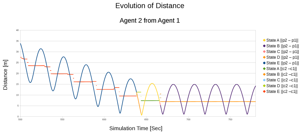
Figure 4.4: A simulation for a 2-agent system with parameters R = 6[m] , r = 4[m] , \alpha = \frac{\pi}{3} and v = 1 \frac{[m]}{[Sec]} . Evolution of both \|p_2(t) - p_1(t)\| and \|c_2(t) - c_1(t)\| is shown, the different colors represent the different states the agent is in with regards to a point half way towards the other agent.
